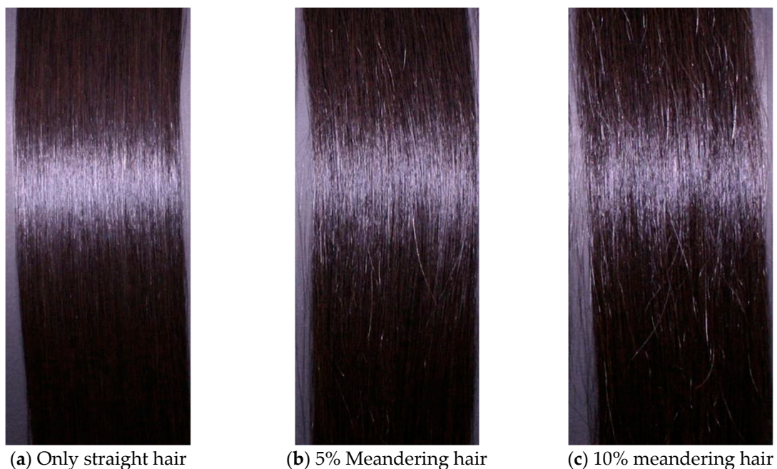
Figure 4. Appearances of hair bundles made from straight and meandering hair fibers. Hair bundle (a) was made from only straight fibers, (b) was from the mixture of 95% straight and 5% meandering fibers, and (c) was from the mixture of 90% straight and 10% meandering fibers. Change in fiber alignment is clearly observed from more- to less-synchronized along hair length, from (a) to (c).
