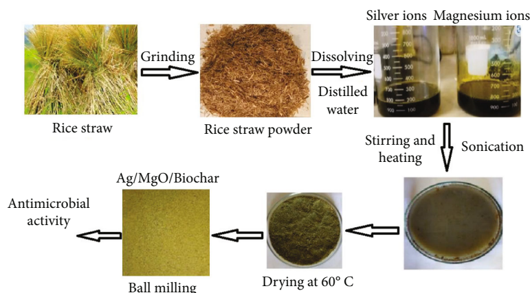
FIGURE 1: Fabrication of Ag/MgO/biochar nanocomposites.
