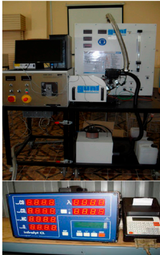
Figure 1. Photo of experimental set-up for engine and gas analyzer.
