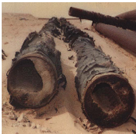
Figure 2. Calcium carbonate \text{CaCO}_3 scale precipitation inside production pipes [13].
