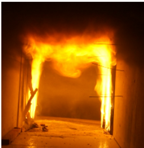
(c) Experimental flame shape at 447 s
