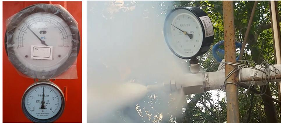
**Fig 13. Comparison of pressure gauge readings.** (a) Pressure gauge reading of tank, (b) Pressure gauge reading at pipe end.
