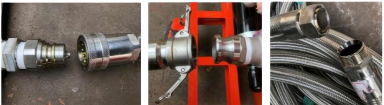
**Fig 5. Quick connection type selected for liquid confluence and delivery.** (a) Self-closing type, (b) Wrench type, (c) Arc surface seal type.
