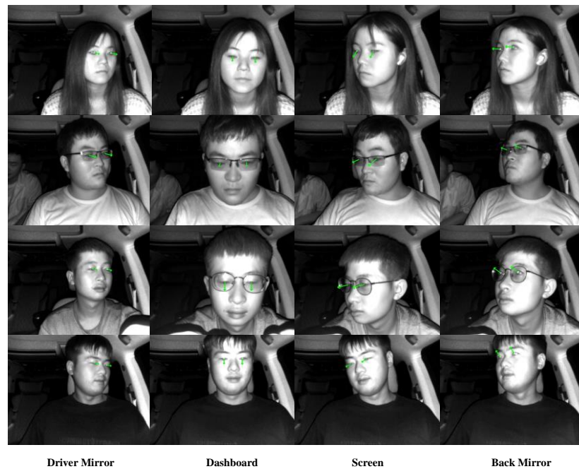
Figure 19. Detection results of driver's partial gaze points in the interior of a Toyota business SUV. Green arrows indicate the driver's gaze direction detected by our gaze-estimation model.
