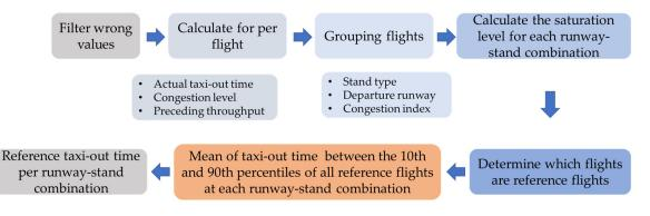
Figure 4. EUROCONTROL PRU method for determining unimpeded taxi-out time.
