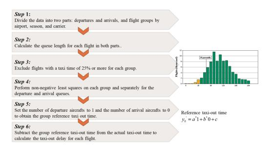
Figure 3. FAA APO method for determining unimpeded taxi-out time.
