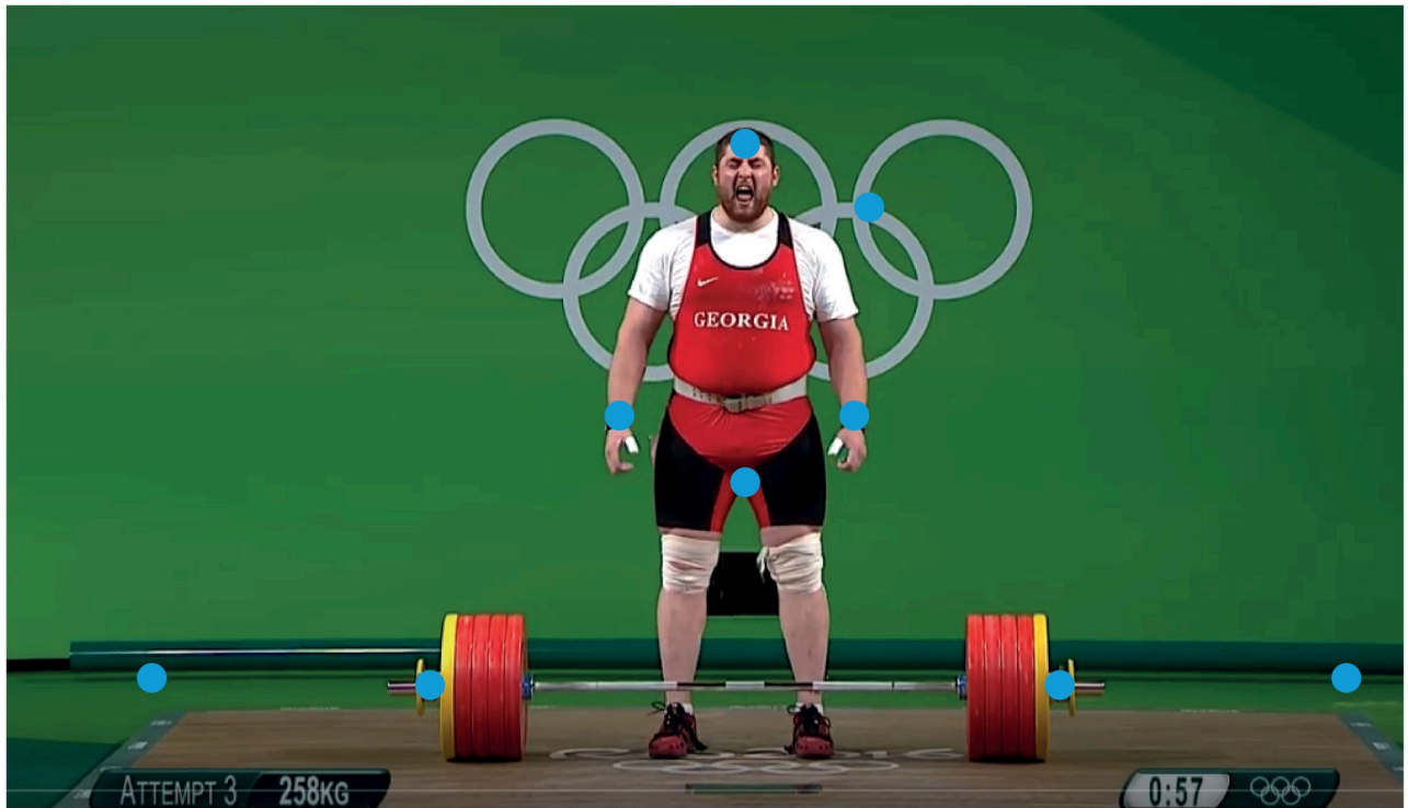
Fig 31. Lasha Talakhadze in men's weightlifting. The video tracking was based on 9 points of interest represented by blue markers, including 3 fixed points of calibration, 2 points on the barbell and 4 anatomical points (forehead, crotch, wrist on the left, wrist on the right). Source of the original video: [25].
