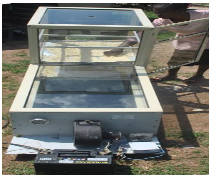
Fig. 2. Experimental set-up showing cassava grates drying process
