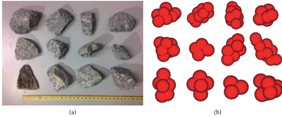
FIGURE 1: Ballast particles and constructed elements of ballast in DEM. (a) Real ballast. (b) DEM model of ballast particles.
