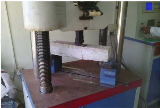
Fig. 3. Specimens undergoing flexural test
