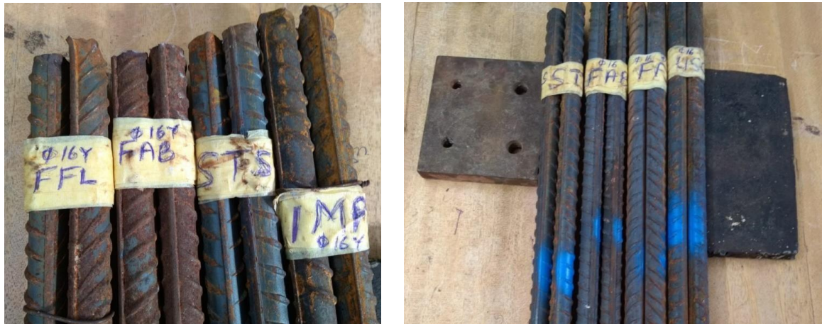
Fig. 1. Typical labeled bar specimens
