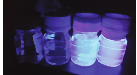
FIGURE 1: Light is emitted from samples illuminated by a 250 nm wavelength UV lamp for eye inspection. From left to right, pure water (H 2 O), 2-ethoxyethanol, NE3, and R sample. Pure water and 2-ethoxyethanol do not emit light. Our main NE3 sample emits a relatively moderate amount of light compared with the R sample at the rightmost vial in the figure.
