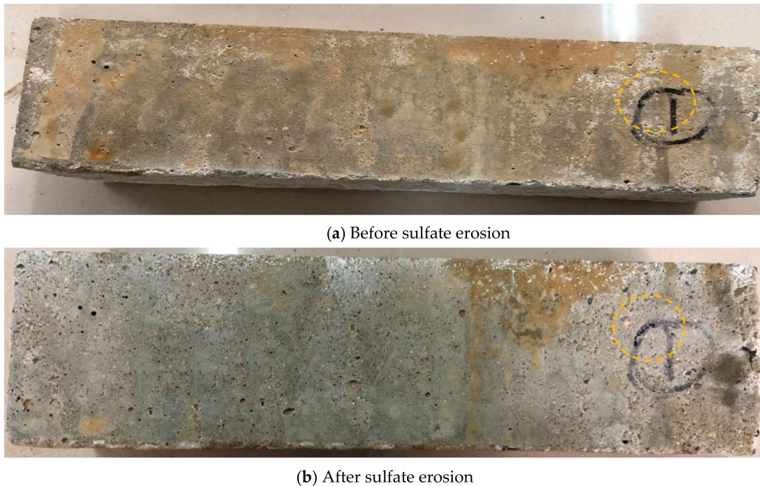
Figure 5. Visual inspection of concrete with dry-wet cycles. (a) Before sulfate erosion; (b) after sulfate erosion.
