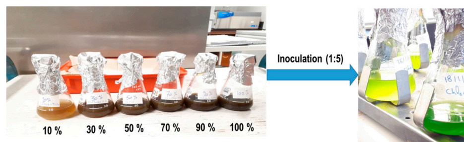
Figure 1. Various diluted samples of anaerobically digested CM (10 to 100%) used for microalgae cultivation experiments.
