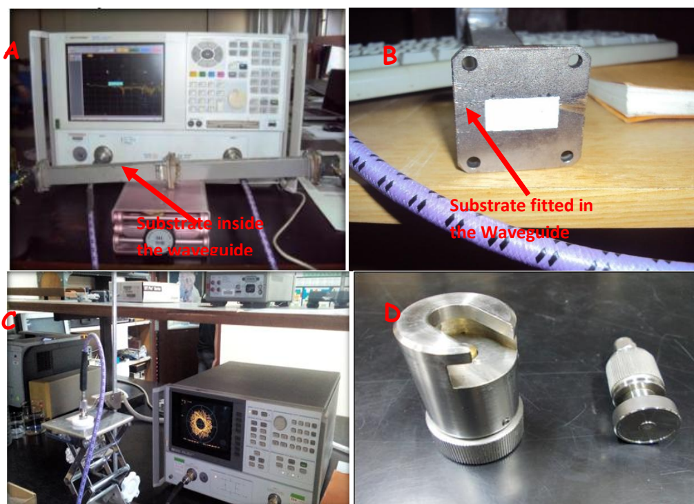
Fig. 1. Measurement Set-up for (a) T/R Coefficients (b) Sample fitting (c) Complex permittivity (d) Shorting Block and Probe Sensor
