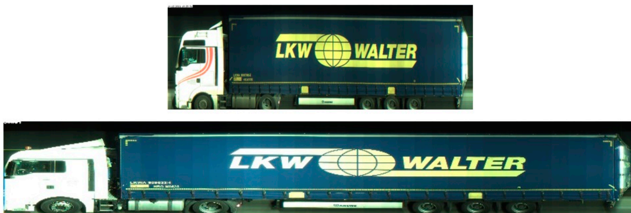
Figure 2. Examples of variable image sizes depending on the truck speed at the OCR gate.
