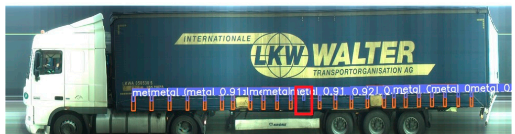
Figure 7. Example of metal parts and whole belts detected by NN2 and NN3.
