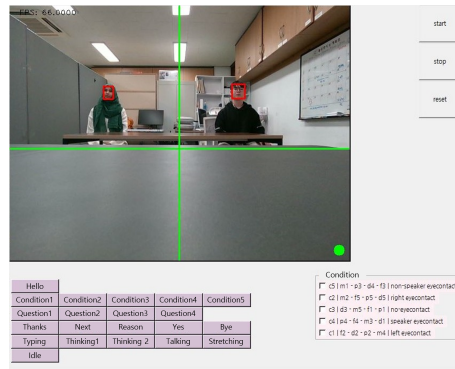
Figure 1. Graphical user interface used in Experiment 1 to control the gaze behavior of the virtual human. The red boxes indicate the participants’ faces.
