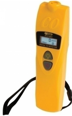
Fig. 1. Picture of the carbon monoxide detector
