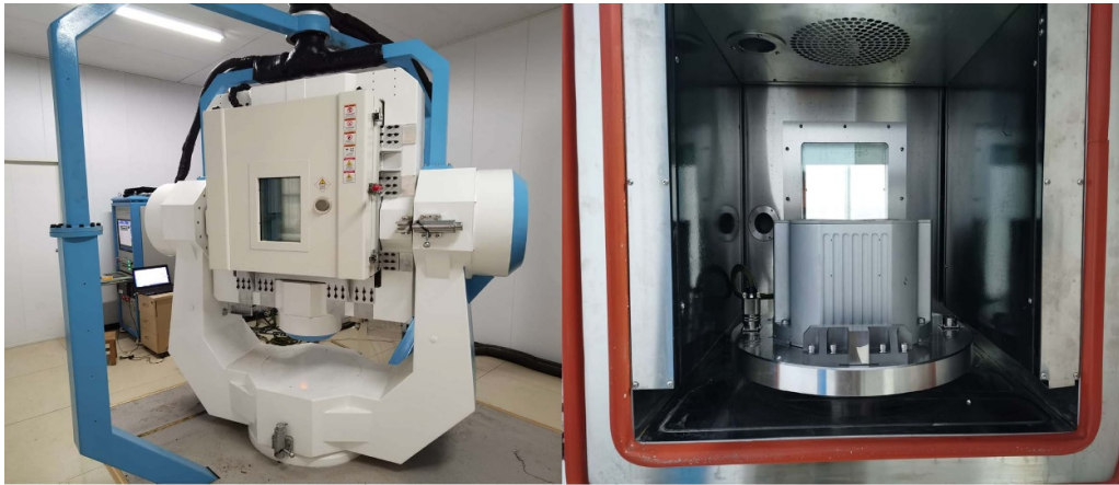
Figure 3. The three-axis turntable with thermal chamber and the IMU for the calibration experiment.
