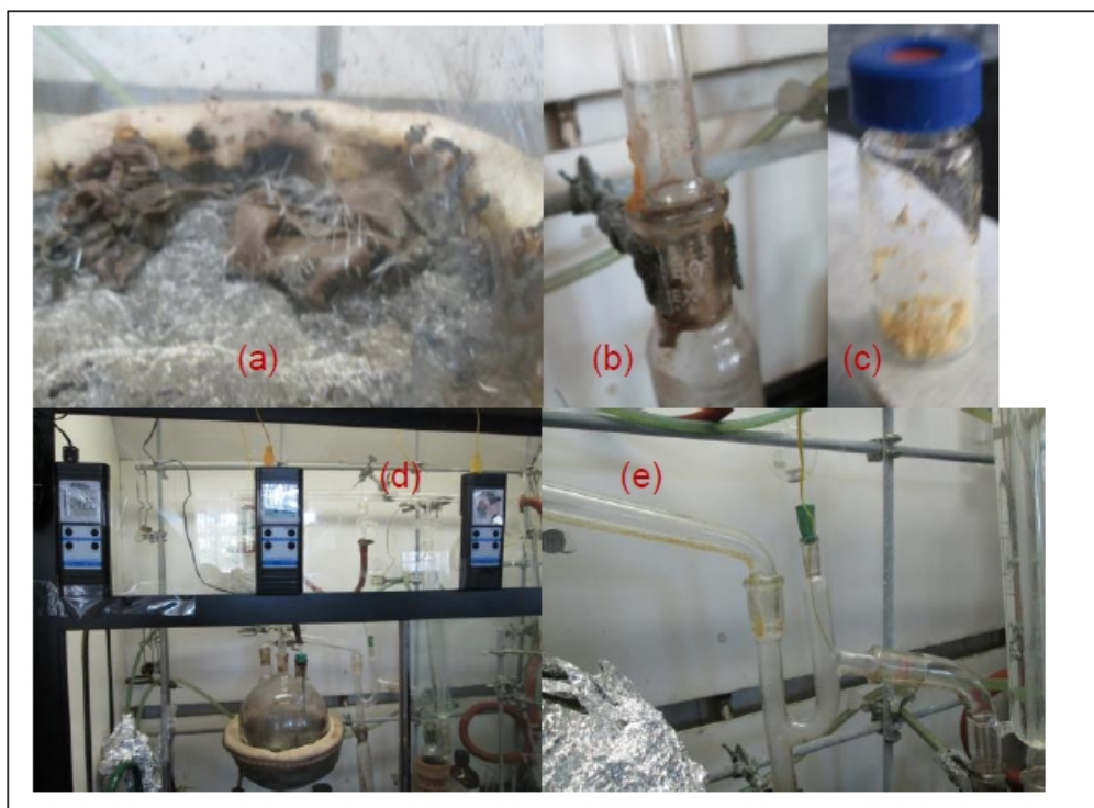
Fig. 2. Step-by-step illustration of the decomposition process of LEGs: (a) the white needle shaped crystals grown in tope of the cold residues, (b) accumulation of solids out of the joints, (c) a sample of the solids, (d) the setup and (e) the condenser with solids
