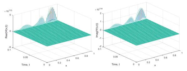
Fig. 4. Real and imaginary part of the central difference numerical solution to equation (6) with  $x_0 = 0$ ,  $x_n = 1.0$ , h = 0.01 at  $t_0 = 0$ ,  $t_m = \frac{1.0}{10} = 0.1$ , k = 0.001, where m = n = 100 & r = 5.0
