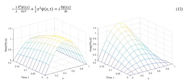
Fig. 2. Real and imaginary part of the central difference numerical solution to equation (3.55) with  $x_0 = 0$ ,  $x_n = 1.0$ , h = 0.1 at  $t_0 = 0$ ,  $t_m = \frac{1.0}{5} = 0.2$ , k = 0.02, where m = n = 10 & r = 1.0
