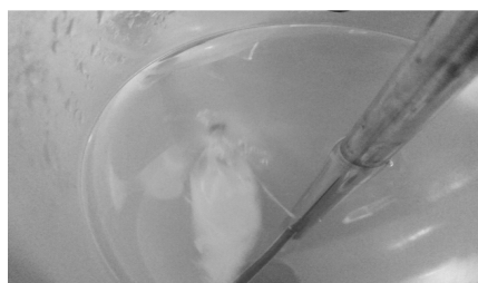
Dialysis sac put in to dissolution vessel
