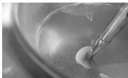
Chicken intestinal membrane put in to dissolution vessel
