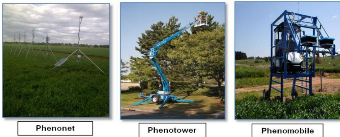
Fig. 6. Field phenomics equipment Source: Roshni and Prajwala [34]
