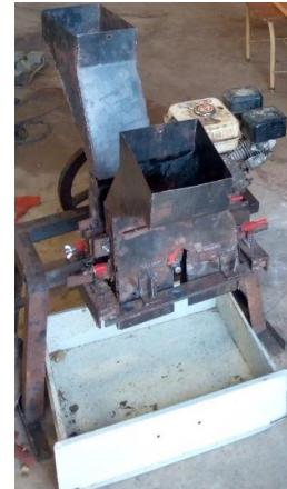
Fig. 2. Operating the dual compartment ginger slicing machine
