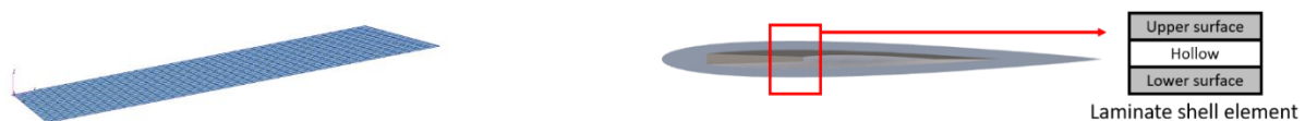
Figure 9. Finite element model (left) and cross-section description of a hollow element (right).
